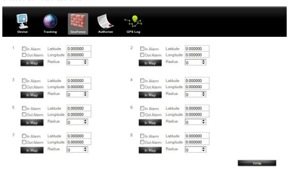
The GeoFence is a circular fence centered at a point with the radius being of a present distance. The maximum number of fences is 8.
